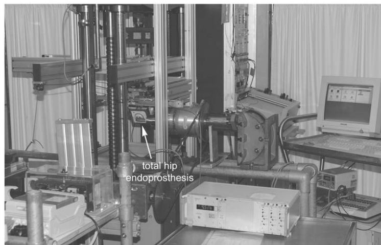
Figure 2 Dislocation testing setup with measurement device and movement actuator in the lateral view, mounted in a universal testing machine. Examined movements: maximum internal and external rotation combined with 90° flexion and 0° adduction.
